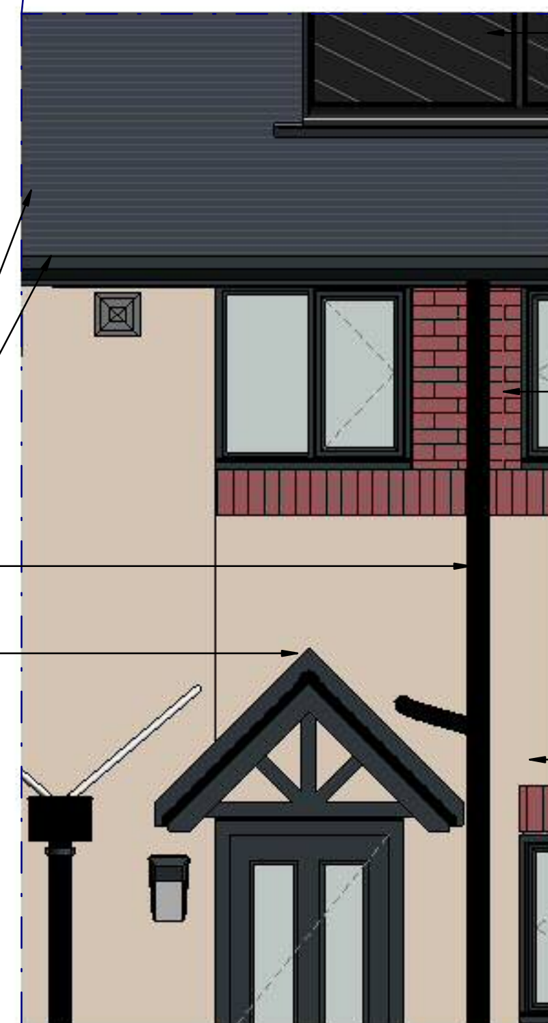
Inline Photovoltaic panels to reduce electricity costs, Marley Solar Tile M10, to be installed as per manufacturer's specifications.
